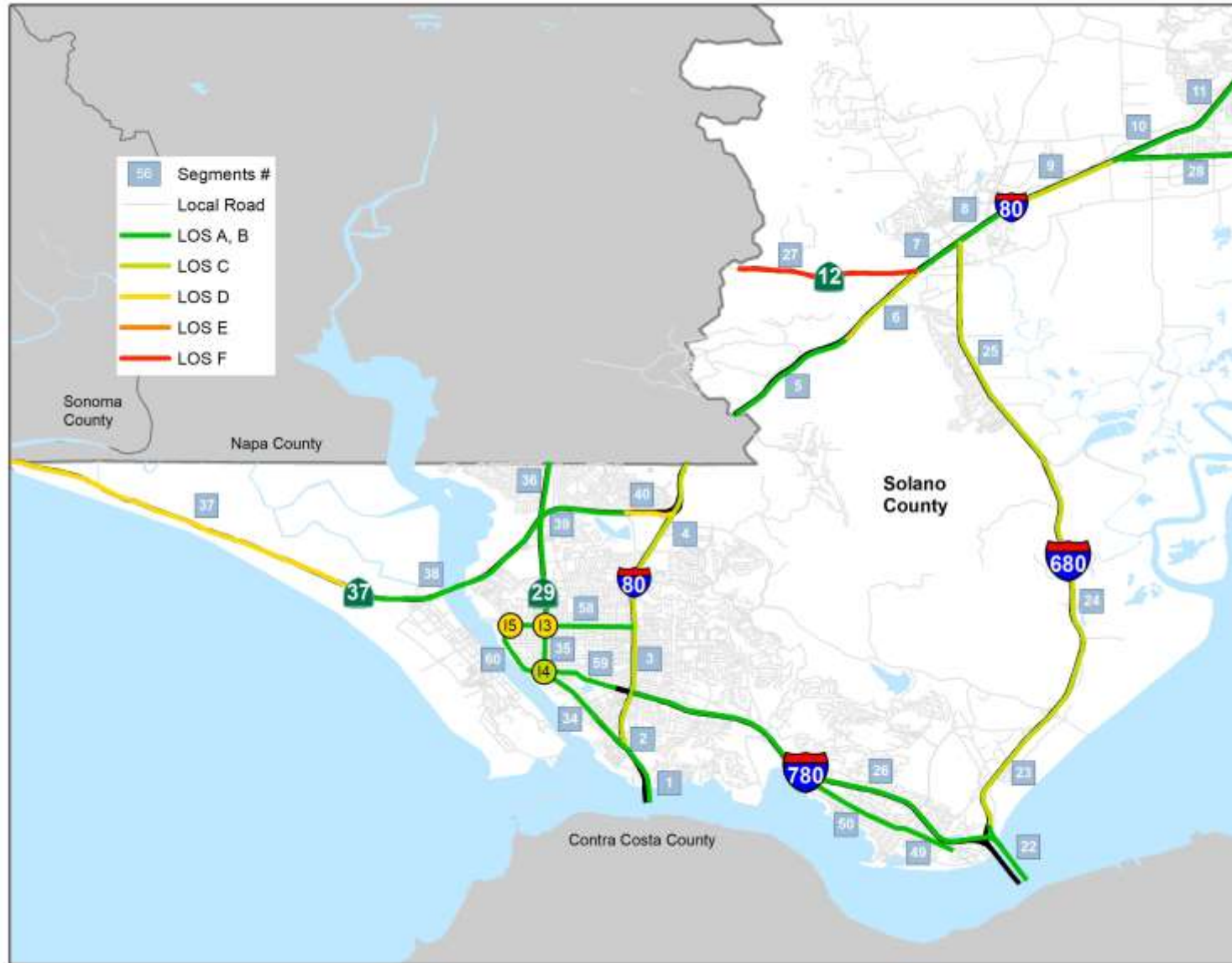
Figure 5 Segment LOS 2023 – South County
