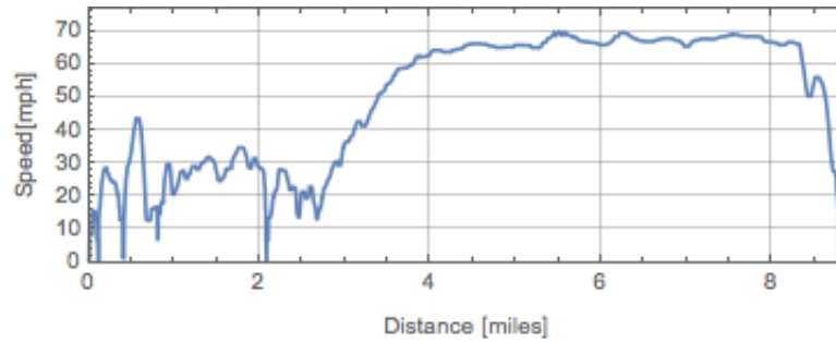
Figure 27. Representative duty cycle for a drive from Suisun-Fairfield to Vacaville
