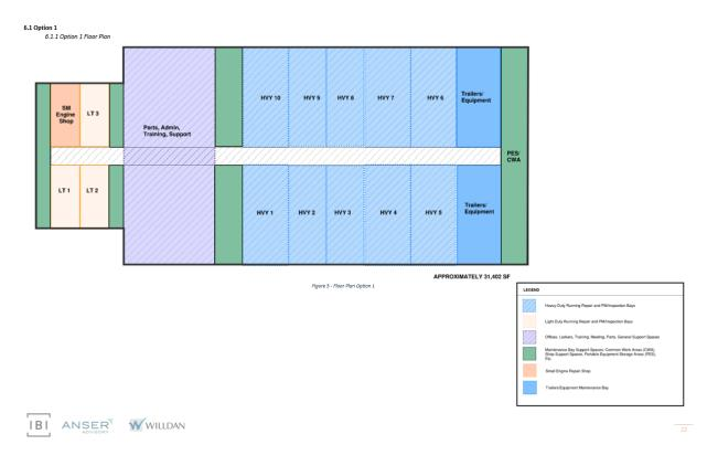
Figure 3. Mockup of New 15 Bay Maintenance Facility (Option 1)
