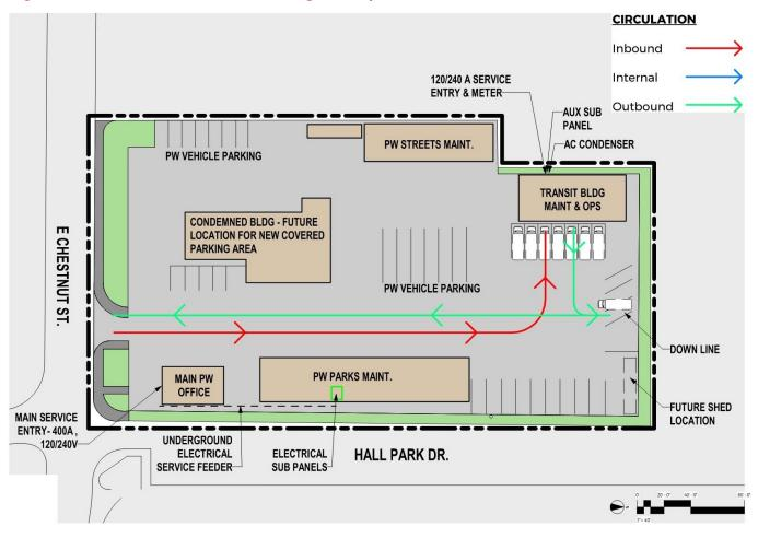
Figure 5.2 Dixon Readi-Ride Existing Facility and Site Circulation
