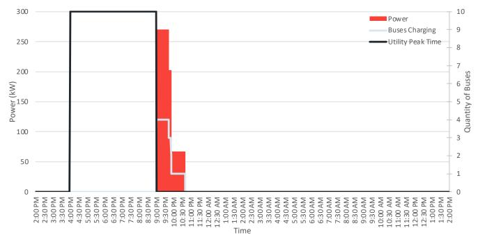
Figure 5.2 Rio Vista Delta Breeze Existing Fleet Unmanaged Charging Scenario: Four Cutaways
