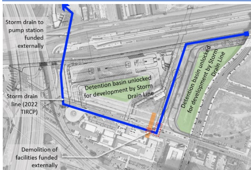
Figure 15: Storm Drain Line and Related Impacts
