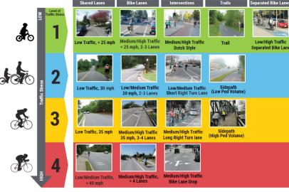
Figure 2. Level of traffic stress by bicycle facility
