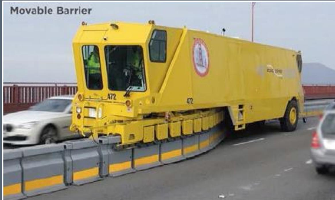
Golden Gate Bridge: Contraflow Lane
